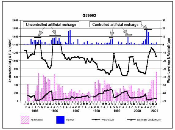
Figure 27: Water level response to artificial recharge at Karkams (Murray 2004a)
