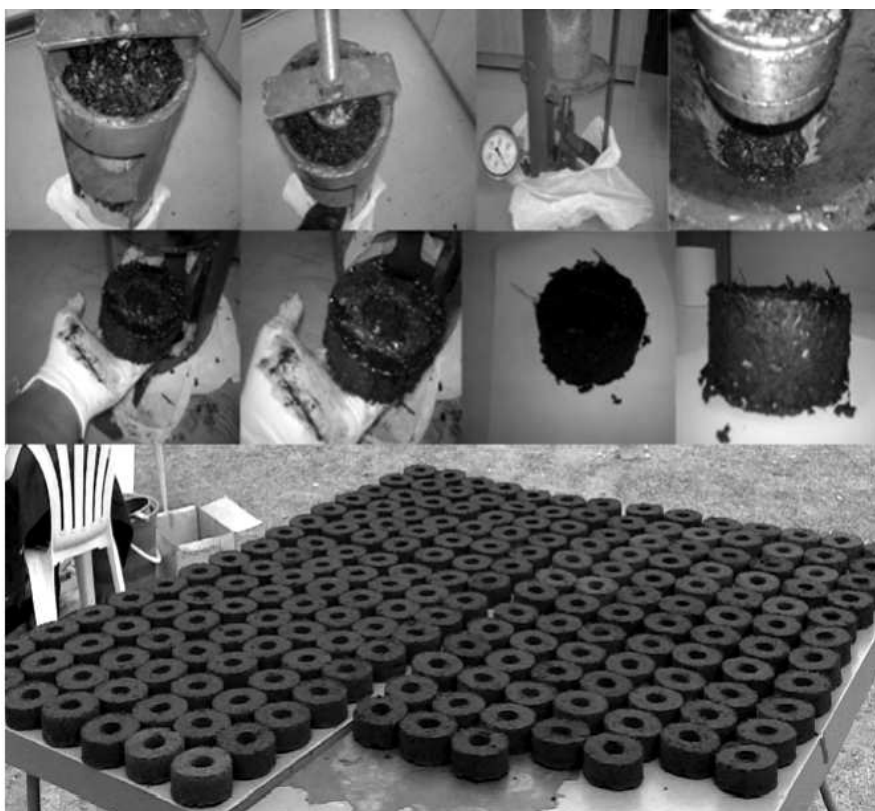
Figure 1: Production of briquettes using a manually operated screw press
