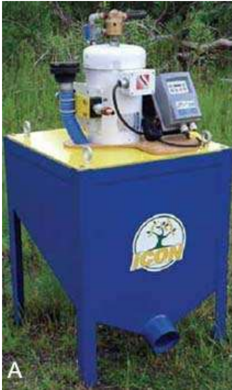
Picture 8. a) Example of an Icon TM centrifuge b) Example of a shaking table used in a small-scale operation in Mongolia.
