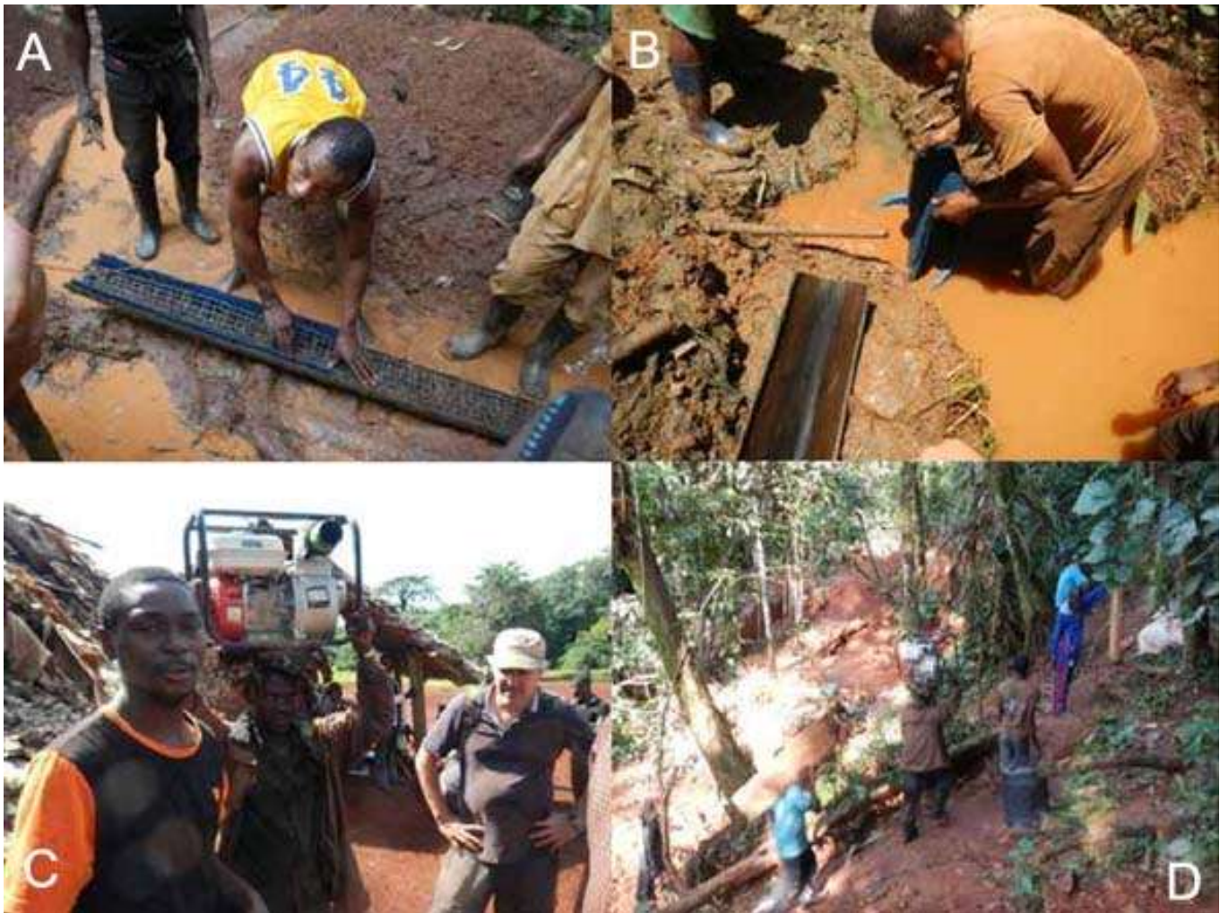
Picture 6. a) Miner experimenting with miners moss on primary sluice. b) Miner washing the carpets. c) Purchase of 6 HP engine. d) Transport of engine to mine site.
