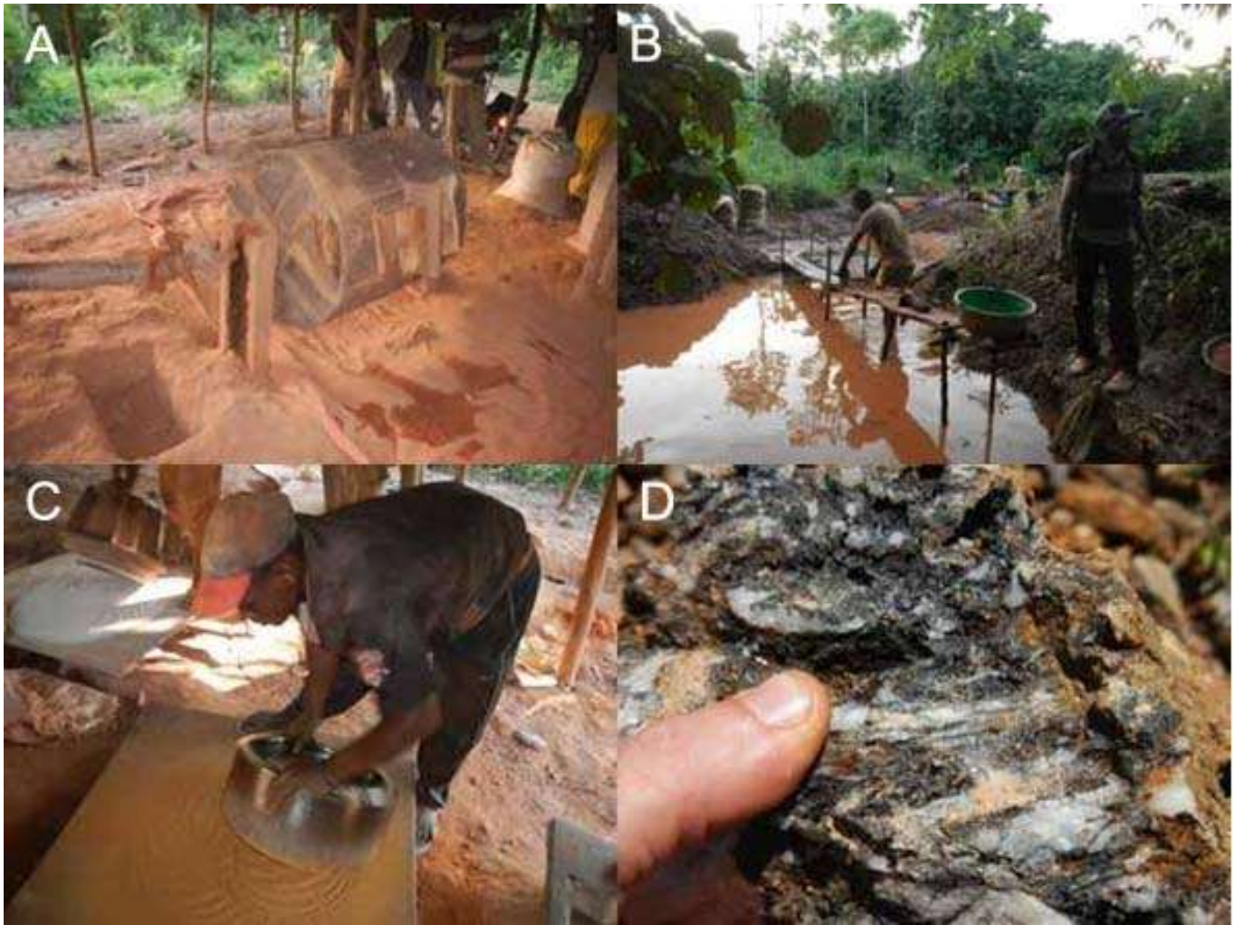
Picture 4. a) Octagonal mill. b) Miners on site c) Crushing and milling to very fine fraction. d) rock with visible gold.
