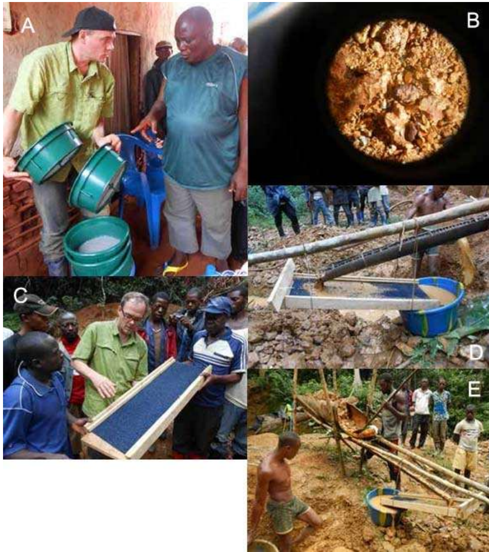
Picture 5. a) Gold sorted through sieves. b) soft matrix of the saprolite in muds clinging to stones and rocks where gold at Mangi is hosted. c) Second or scavenger sluice with miners moss brought from Canada. d) Zig zag sluicing on site. e) Miners using the zig zag sluicing.
