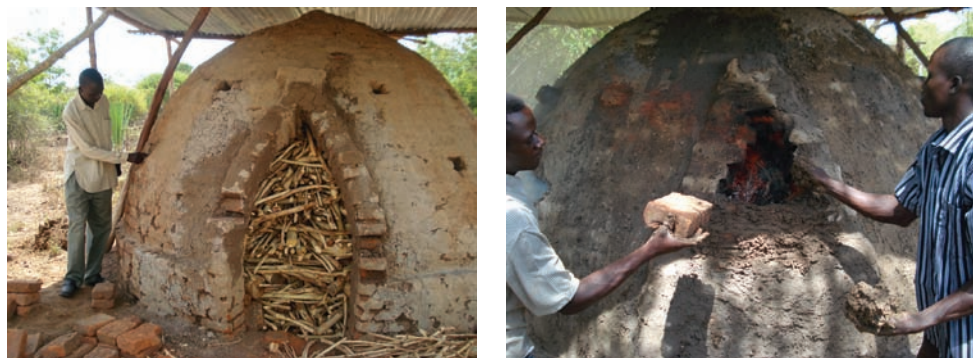
Left to right: Wood arranged tightly inside the half orange kiln, and sealing the door way of the kiln (Nellie M. Oduor, KEFRI).
