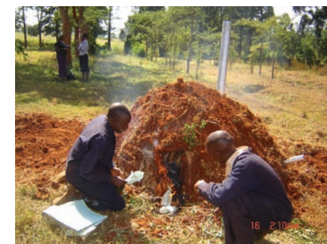
Right: Lighting the Casamance kiln after covering the wood. The metal chimney is visible at the back of the kiln (Nellie M. Oduor, KEFRI).
