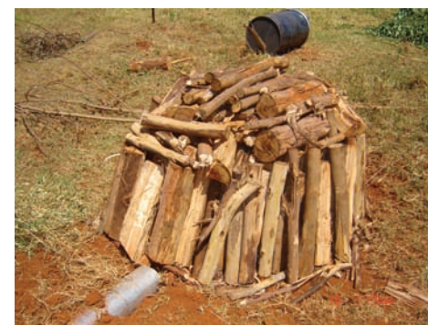
Left: Wood arranged upright for Casamance kiln (Nellie M. Oduor, KEFRI)
