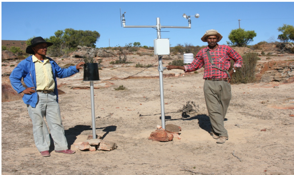
Figure 10: Weather station on Dobbelaarskop, with Koos and Hendrik Hesselman after installation. Photo: B Koelle
