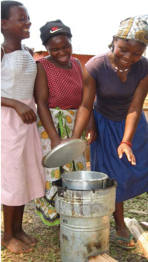
Figure 8: More efficient and healthier use of fuel wood (metal type, portable, outdoor); compared to Figure 4.
