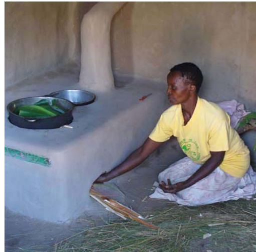
Figure 9: More efficient and healthier use of fuel wood (clay type, fixed, indoor kitchen); compared to Figure 4.
