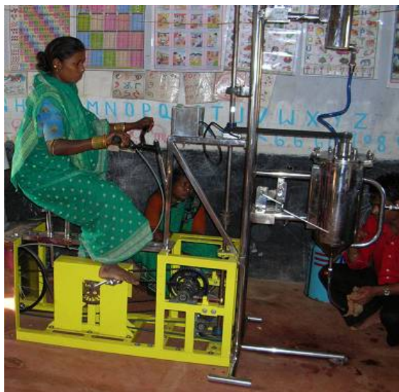
Pedal-driven biodiesel reactor (Photo: CTxGreEn)
