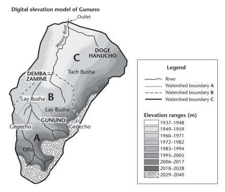
FIGURE 3.1 Digital elevation model illustrating hydrological boundaries and features of Gununo watershed, Ethiopia
