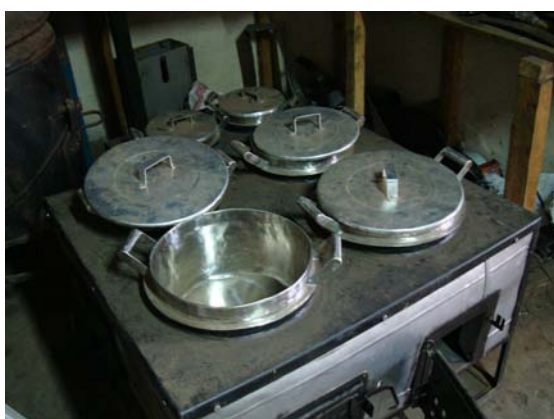
Example of an energy saving Institutional stove with fitted pots developed by Mussoo Engineering on display at Kisumu. Mussoo is an income generating initiative implemented by a youth group in the urban and rural areas of Kisumu, Nyanza and Baringo districts
