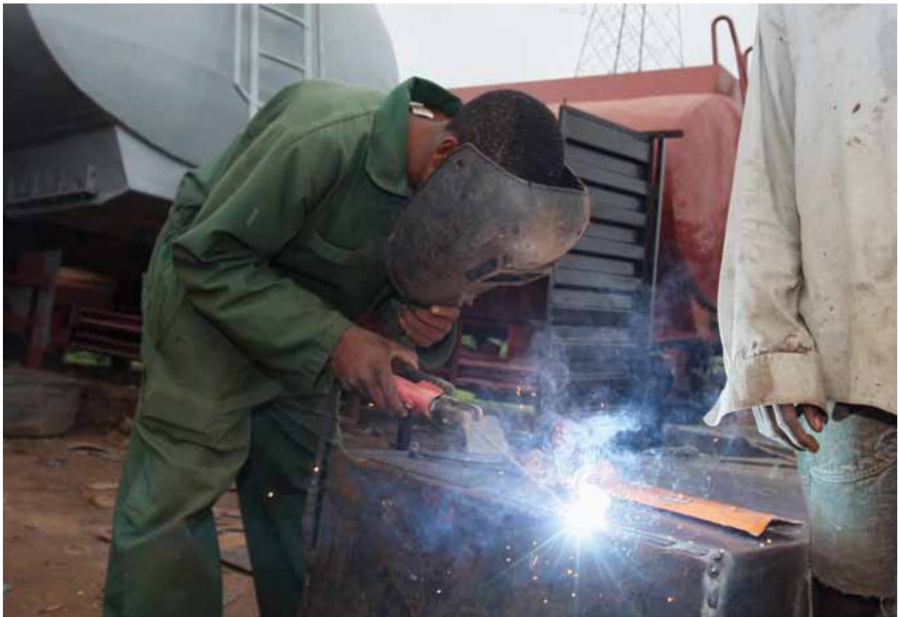
Men construct petrol tankers at the side of the road on the outskirts of Lagos, Nigeria. The workers have as many as ten tankers on the go at any one time, taking about one month to construct each one.
