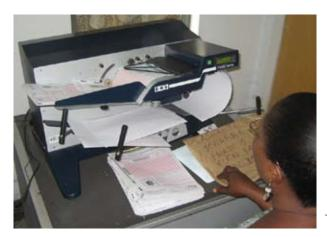
Despite the fact that vendors quote a higher rate, the practical experience of Ghana is that the scanners can process about 1,000 forms an hour in real working conditions.
