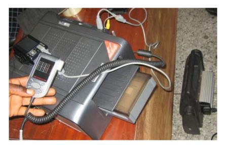
New technology: Data from the digital camera is transferred to the printer via a cable, and the colour printer produces up to eight pictures on the spot.
