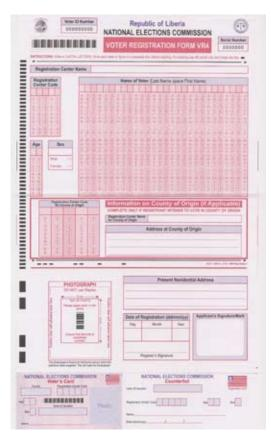
Form used in Liberia in 2005: Personal data is captured using ICR and OCR technology and barcoding. The form features pre-printed serial numbers and spaces for the applicant's photograph, signature and fingerprint.
