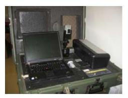
The second generation registration kit used in Ghana comprises a computer, a digital camera and a printer. The first generation kit used a Polaroid camera.
