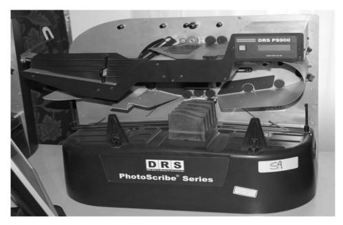
The scanner uses combined OMR and image recognition technology. It can detect and record – in real time – a variety of items on a form including the barcode and photograph.
