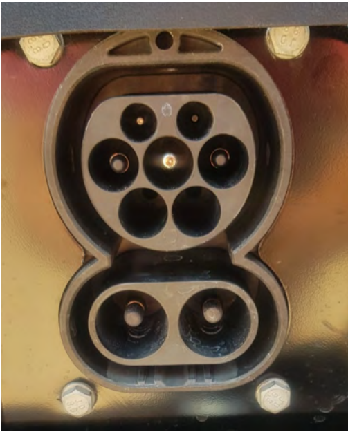
Figure 11 A CCS DC fast charging port on a 48 kWh BYD T3 Van in Harare
