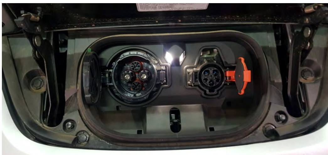
Figure 10 A Chademo DC fast charging port on a 62 kWh Nissan Leaf e+ in Harare
